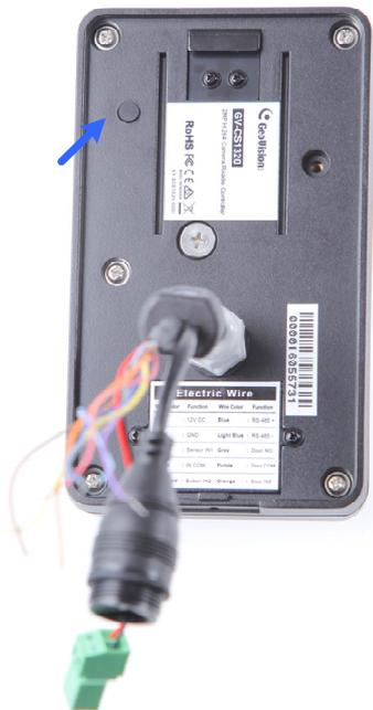
3. Wait until the status LED blinks twice to release the **Load default** button. The process takes about 5 seconds.
